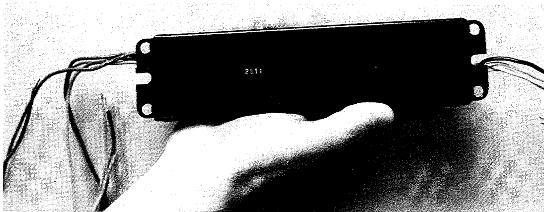
Photo 6c. Example of a Manufacturer's Date Code. The first two digits on this date code must be reversed to determine the year of manufacture. This CGE ballast was made in November (11), 1982 (28).
