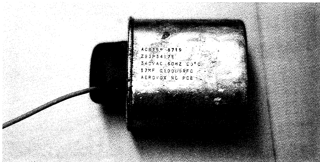
Photo 4 Ballast Capacitor. An Aerovox capacitor with NO PCB stamped on the can. The label markings indicate that this capacitor was made in the 19th week of 1987.
